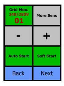
Auto Start - If enabled, forces charger to stay ready to charge even if not plugged, unplugged from car, stopped from the car. No need to start charging every time. **It must be off for firmware update.**
